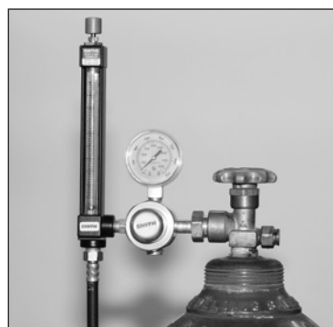
Figure 4.15 The regulator/flowmeter regulates the flow of shielding gas from the cylinder to the welding torch. This meter displays the amount of pressure in the cylinder as well as the rate of flow.
