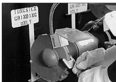
Figure 4.10 Tungsten electrode preparation.
