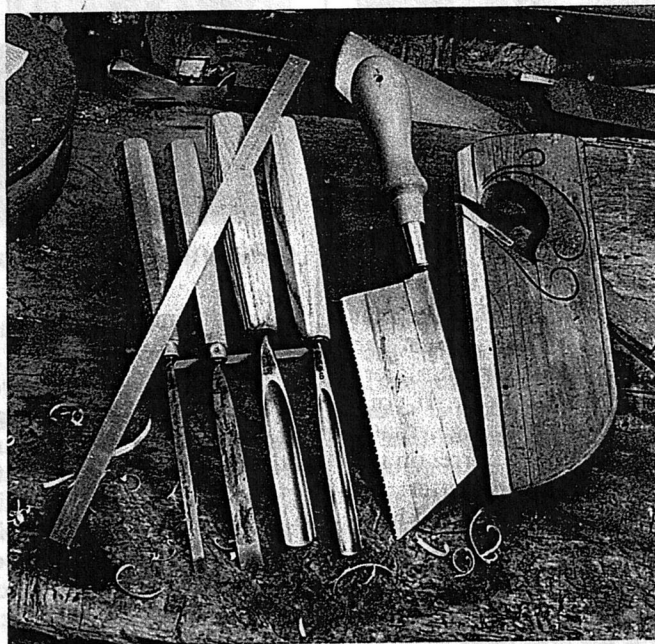
The tools of the job: chisels, gouges, a modified back saw, and a warmed-over rabbit plane which will be discussed in the next issue.
