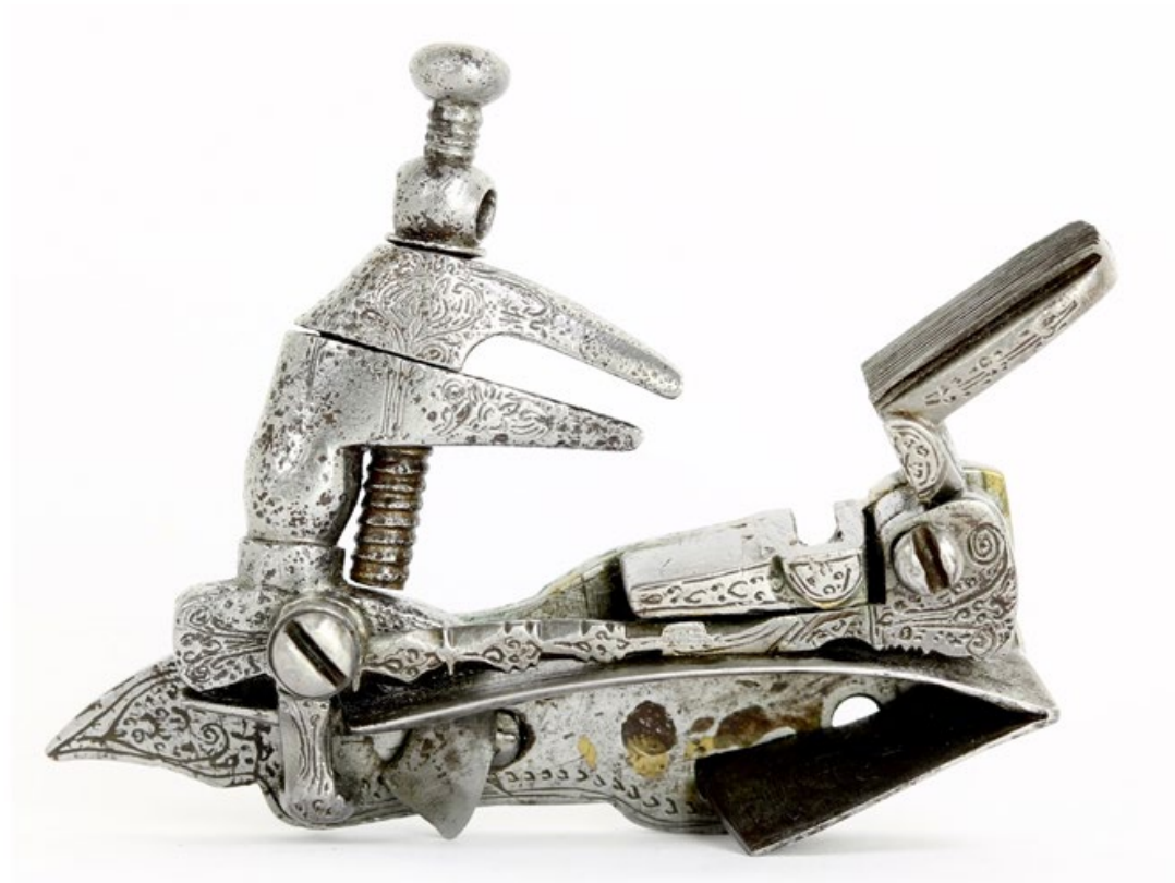
Balkan miquelet after being triggered, with pan cover open.
