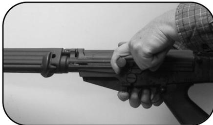
4. Grasp the cocking lever and pull it to the rear of the rifle and allow it to snap forward. Pulling the cocking lever to the rear releases the bolt hold open device which allows the bolt to travel all the way forward. (Do not "ride" the cocking lever forward by continuing to hold it, slowing its forward movement, as this can prevent the bolt from closing properly and prevent the extractor from engaging a cartridge which has remained in the chamber.)
