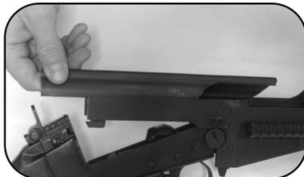
Separating the Upper Assembly from the Lower Assembly Unscrew the hinge bolt and remove it. The upper assembly will separate from the lower assembly (See Illustration #21).
