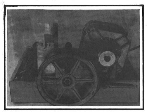
This is the mill base. It consists of a frame, electric motor, pulleys and rollers. The smaller pulley is the one you need to change to adjust rpm. This model will hold two 6 pound drums.
