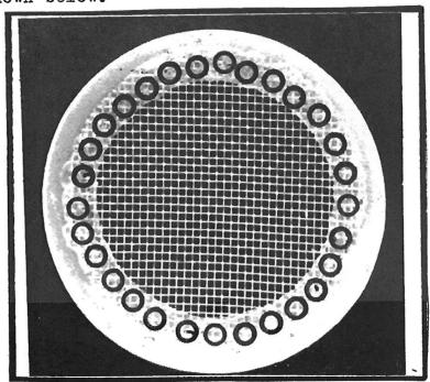
Step 5. Tack down the inside edge and any wire screen ends, as shown below.
