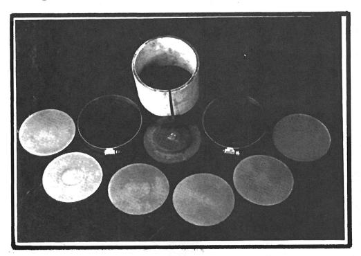
Also shown are the bowl bottoms that have been cut out of the Rubbermaid bowls. These bowl bottoms are used for spacers, along with the pressing plate. You will need eleven bowl bottoms.
