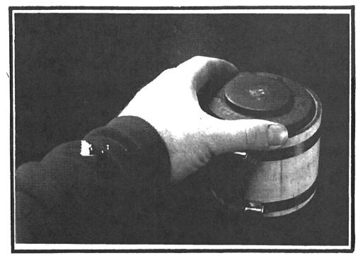
Taking the completely assembled pressing sleeve, turn it upside down with the pressure plate now on the bottom and place into the hydraulic press and add pressure; see the photograph below.
