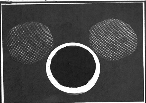
cut to fit on the inside. Between the two screens, you place one sheet of toilet tissue to act as a filter to let air in and out at the same time retaining the black powder grains.
