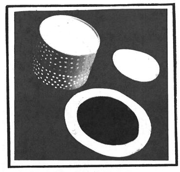
The Rotary Separation Mill, the ring and the bottom to hold it in place. In the photograph shown below, we show a 1/8" Rotary Separation Mill having it's bottom hot glued into place. We used three passes of hot glue.
