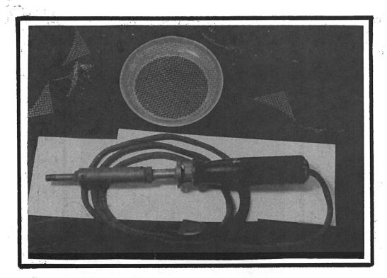
cut to size and placed in the bowl bottom. This soldering iron has a blunt end to transfer the heat more evenly.
