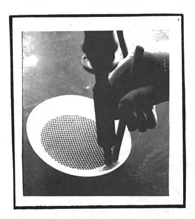
plastic bowl bottom. Remove the soldering iron slowly, while holding the dowel in place. When the plastic cools, it will hold the screen in place.
