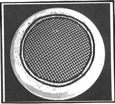
Here is a completed bowl mounting ready for use. A dye has been added to show the areas of adhesion.
