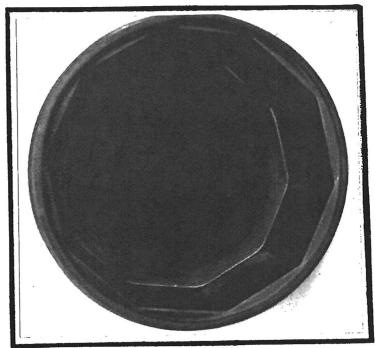
The inside of the mill drum should have 6 to 12 sides. The sides help in turning the powder and the balls over as it rotates.
