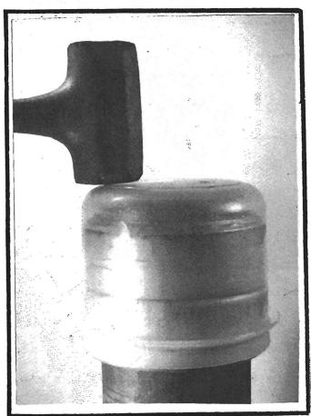
a hard plastic mallet (shown on previous page), where the bowl sets on the cutting edge. Warming the bowl will help soften the plastic so that it is more easily cut. This can be done by running hot tap water into the bowl just before cutting.
