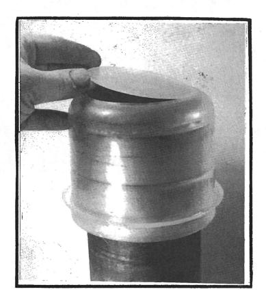
As you can see here, the bottom is cut very precisely with this technique and the bowl bottom is easily removed. You can remove the bowl bottoms of about a dozen bowls in just a few minutes.
