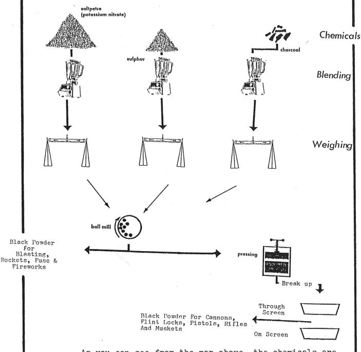
As you can see from the map above, the chemicals are first pulverized and weighed, then placed in a ball mill. When they are removed from the ball mill, this powder can then be used for a number of chemical projects, or you can further refine this powder into high density grains for use in black powder firearms; see Section Two.
