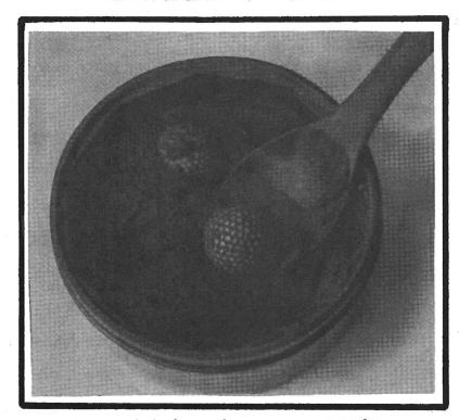
For safety's sake, use a wooden spoon to remove the balls after the milling to prevent any sparking.
