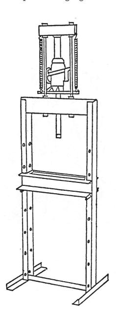
The photograph shown below is of a homemade hydraulic press. This press has a gauge with a maximum pressure reading of 4000 psi. A two ton hydraulic jack has been placed inside. The press body was made out of a piece of eight inch by
