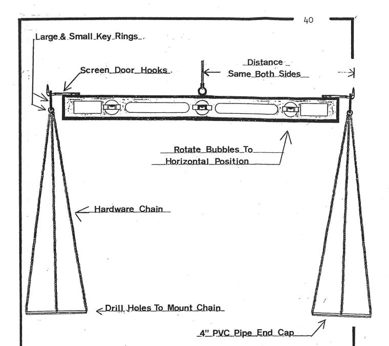
Shown above is a drawing and simple instructions for a balancing beam that we made from a 4 foot carpenter's level.
