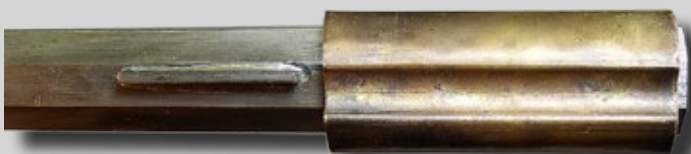
(Fig. 10a) The groove in this cap was formed using a 3/8" diameter steel rod as a counter swage.
