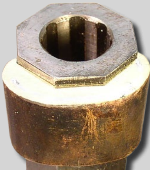
(Fig. 6) Whatever cap forming method you use, pay particular attention to the end plate-barrel fit. The cap-to-barrel fit of this short Jäger cap is about as good as it gets.
