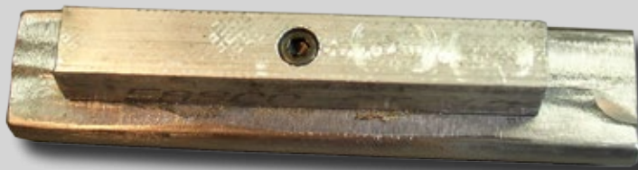
(Fig. 8) A boss on the bottom of this swage for forming grooved two-piece caps provides no-slip clamping in the vise while keeping the sides of the swage free for forming the cap around it.
