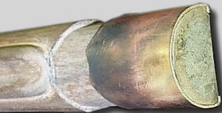
(Fig. 1) Keith has formed the barrel of this muzzle cap, using the fore end as his mandrel. Here he is sliding the cap on to test the fit. When it slides back to the fore end shoulder, he will scribe the outline of the barrel channel on the inside of the end cap and cut that carefully to fit the barrel.
