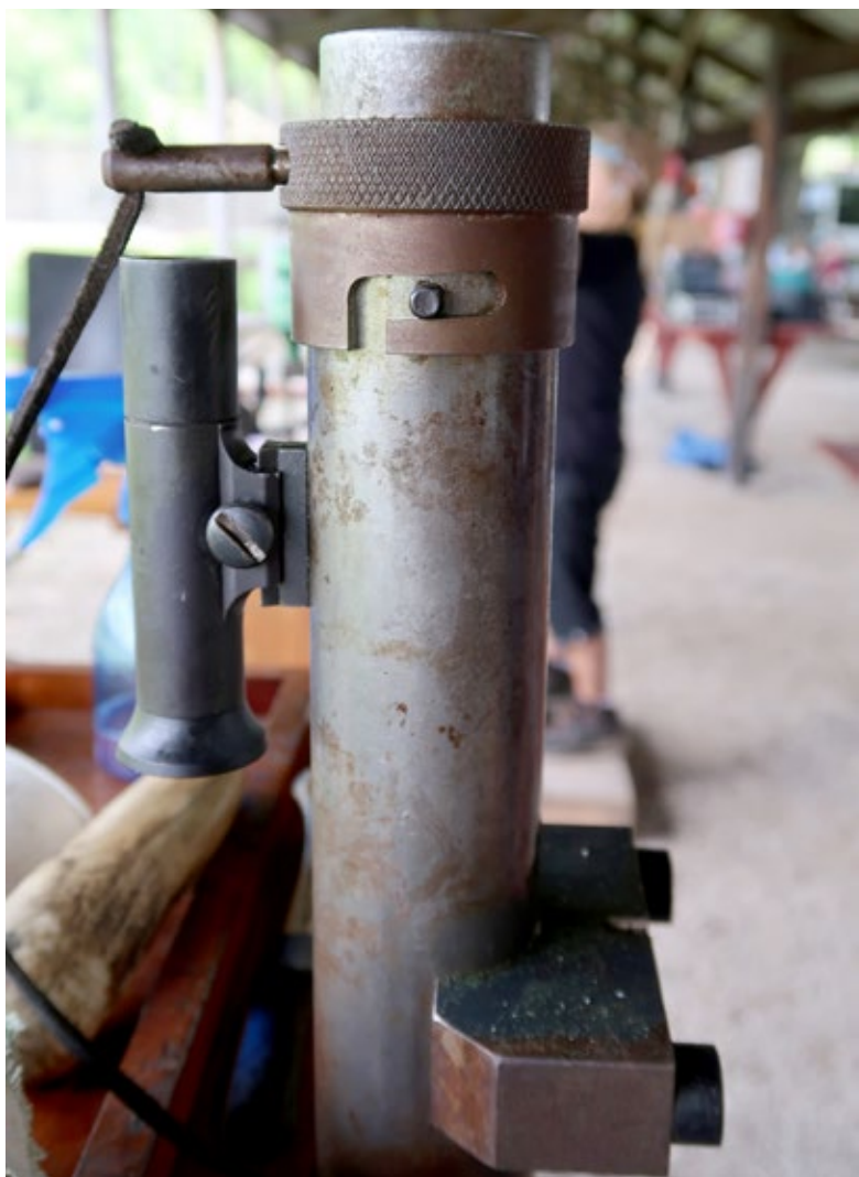
A false muzzle in place for loading. Note the mounted cant block, globe front sight, and safety cord for attachment to the bench to prevent leaving the device in place while shooting.
