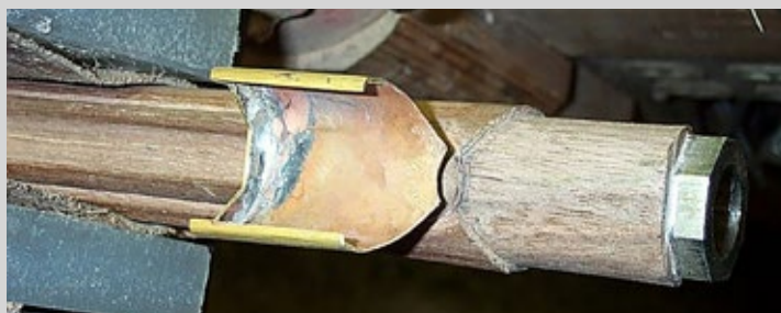
(Fig. 2) Keith reinforces the end plate of his muzzle caps with a sturdy filet of silver solder to support its forward edge that is most vulnerable to damage.
