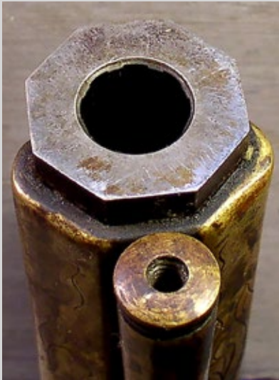
(Fig. 5) You can't tell this is a one-piece swage-forged cap. There is less than 1/8" between the bottom barrel flat and the ramrod. This allows an ultra-slim fore end.
