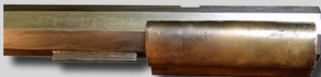
(Fig. 10b) If you shaped the barrel of the cap closely to the barrel, it will hang on even if you shake the barrel.
