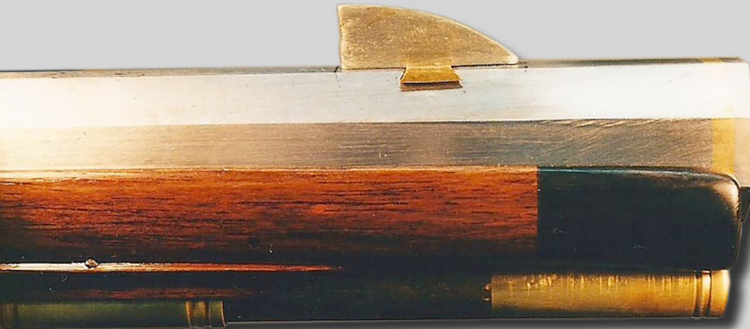
(Fig. 13) Showing more of the barrel accentuates the flare of a swamped muzzle. The illusion works with solid horn muzzle caps too. Note the Nu-Gold muzzle band. It will show up better after browning or bluing.
