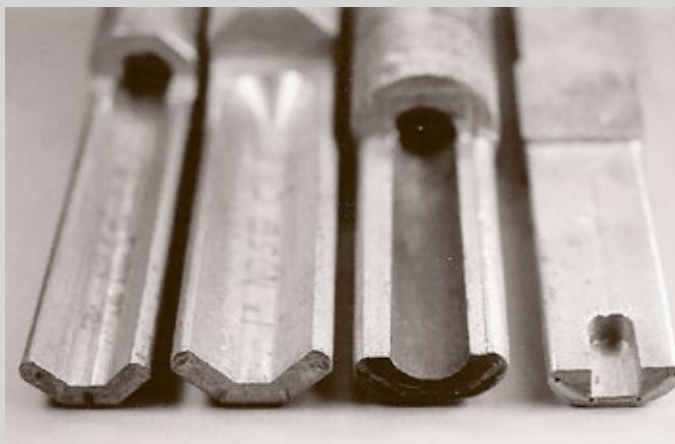
(Fig. 4) Samples of swages for custom-formed caps; some were formed using waste sections of barrels, others were milled from mild steel bar.
