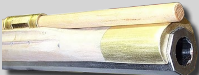
(Fig. 3) A nicely formed and fitted muzzle cap by Keith. Note that the barrel protrudes beyond the cap to allow alignment of loading blocks if desired.
