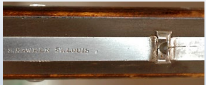
Short rear sight held on barrel by raised lifts. (Gordon, 2007)
