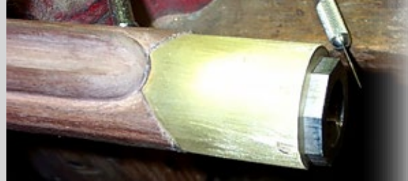
Making a custom muzzle cap for your rifle provides an opportunity for creativity. This cap by Keith Lisle (Custommuzzleloaders.com) is shaped to fit a molding of the stock.
