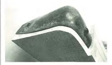
Next I file up the edges as you would for a cast butt plate, when preparing it for inletting. After the inletting is finished, I drill the holes for the butt plate screws and install them.
