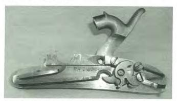
(Figure 1) The Siler lock internals have been around for decades and have proven themselves to be rugged and reliable.
