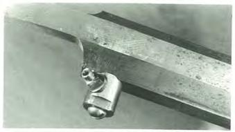
(Figure 3) This drum and nipple system provides a short path to the main charge. The nipple tube has been shortened and chamfered. Nipple placement is as close as possible to the barrel. The drum is countersunk into the side of the barrel.
