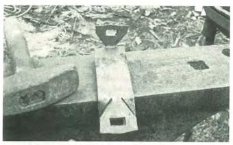
Fig. 4: Once again heating the creeper and bending up the tabs for the thongs and bending down the cleats.
