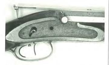
Story rifle lock inlet with the lock removed; note - only one screw (in center) holds the lock to the gun. The only protrusion from the lock is the square post that fits into the square hole in the sear.
