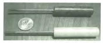
I made my first small flat chisel out of a soft screwdriver. It dulls easily but I would rather have something easily sharpened than so hard you can't sharpen it. The handles are half-
