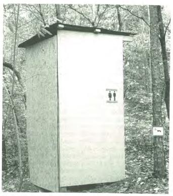
Figure 4 – Our outhouse is sturdily constructed of painted (oil-base exterior) OSB and heavy pine posts set at least 2 feet in the ground.
