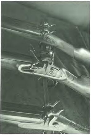
Top to bottom: Cabela's 12 gauge made by Pedersoli with changeable screw in chokes, 20 gauge double flint shotgun imported by Middlesex Village, and 12 gauge original made in Belgium.
