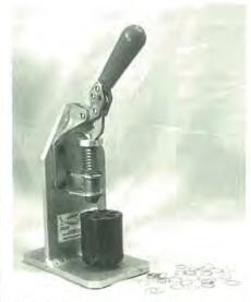
Cylinder loading stand showing the lead rings cut off the balls when they are forced into the chambers
