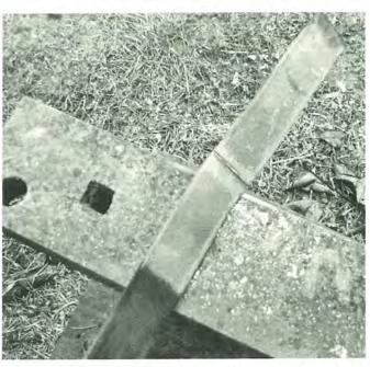
Fig. 1: Heating up the 1  $1/2 \times 1/8$  inch, flat stock in the forge and hammering a crease across its back on the edge of the anvil. Overall length of the stock for each piece is roughly 4  $\frac{1}{2}$  inches.
