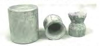
A recovered howitzer projectile and two of our rifle's projectiles recovered from the berm behind the target. The middle projectile is our best. You can see the raised area that expanded into the rifling grooves. The projectile on the right is of a different shape and metal composition and did not work well.
