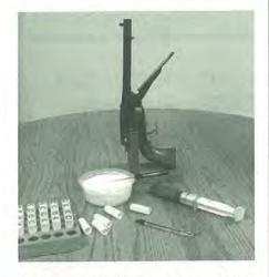
Remington in loading stand with cartridges, filler, lubricant in syringe, and capper
