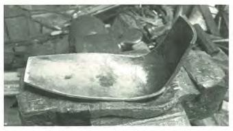
The hammering continues into the heel extension and the plate area. Some bending follows to match the side profile. The metal is quite forgiving. Just keep hammering and checking the shape often. When it looks like a butt plate you are done with the hammer.
