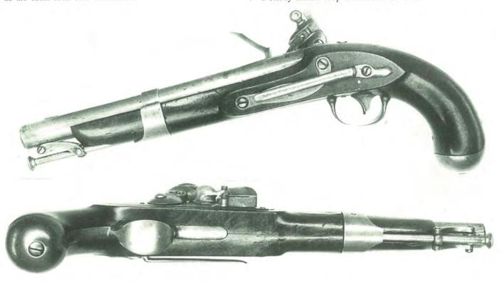
(Figure 5) An 1826 North pistol with a belt hook that has a long flange extension to resist outward leverage on the tang. Note that the hook is not held in place by the rear lock bolt. Photographs courtesy of Dr. James B. Whisker.
