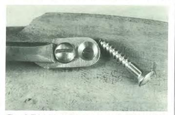
(Figure 7) This belt hook will be inletted and held in place by both the rear lock bolt and a hefty wood screw.
