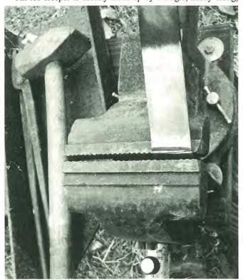
Fig. 2: I was able to break off the size I needed to make the creeper in a vise by moving it back and forth.
