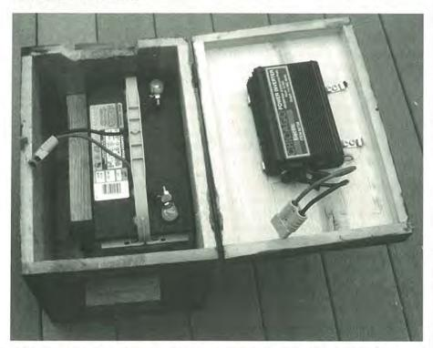
Here is my big week-long system; this was my first attempt at a battery system. I used a 400/800-watt inverter and heavy gauge wires and disconnect. This overkill does not hurt anything, but it is unnecessary. My battery is a 114-amp-hour deep-cycle trolling motor battery. This battery came from Wal-Mart.
