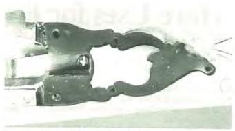
Figure 6. The many little projections of this open-work "island" can be strengthened by epoxy.
