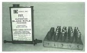
A block I use for cartridges to be tested – Each row of five is loaded with a slightly different powder charge.
