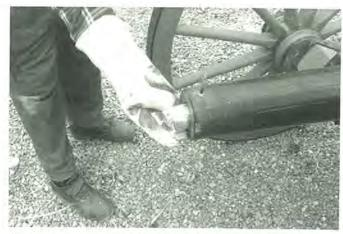
Placing the powder charge into the muzzle
