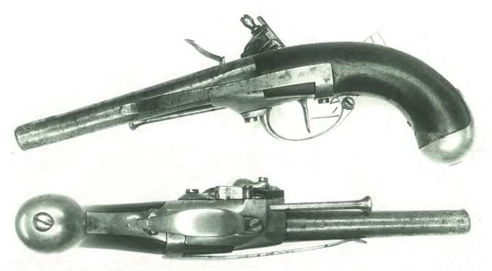
(Figure 3) A French model 1777 naval pistol with belt hook. Note unusual means of attachment. Photographs courtesy of Dr. James B. Whisker. Bedford, Pennsylvania.
