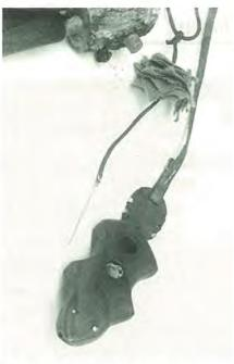
Note cleaning patches "strung" on leather string for quick cleaning. Nipple pick is attached to the end.
