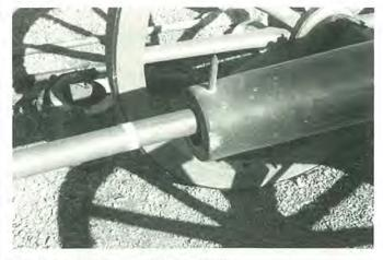
The proper seating depth for the projectile
