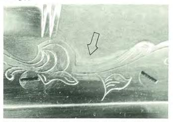
Figure 12. If all epoxy is not removed from around bedded parts, the wood will resist taking water-soluble stains and remain a different color from the surrounding wood.
